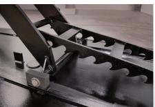
Locks shown in the raised position during lowering of table Compliant with Standards for Garage Equipment - adds additional support and safety guidelines
