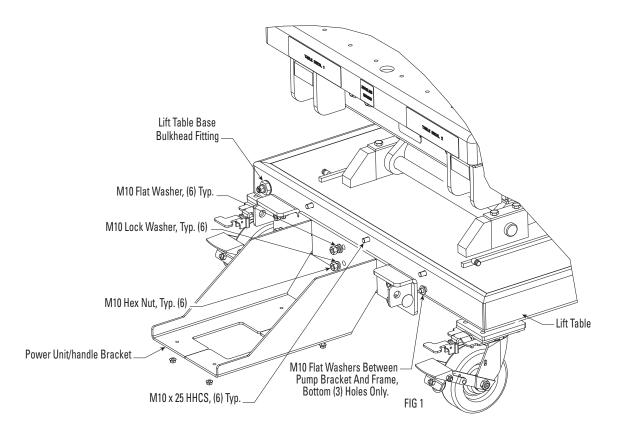
3.) Attach handle to power unit/handle bracket by placing (1) handle pin into the power unit/handle bracket handle hole and then squeezing handle down rods together and inserting the other pin into the other power unit/handle bracket handle hole. After pins have been inserted into holes, place retaining cap over pin, taping into place with a rubber mallet. Lastly, attach springs to the cart spring pin and handle spring pin. Fig. 2.
