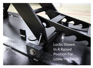
b.) Depress front of foot pedal on power unit until desired height is reached. Review Figs. 3 and 4.
