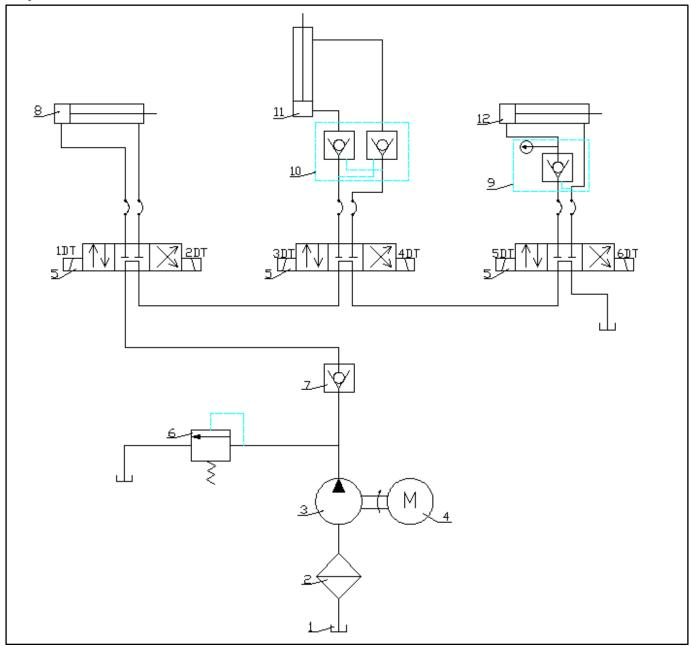
1.oil tank2.filter3.oil pump4.motor5.solenoid valve6.overflow valve7.one way valve8.trailer oil tank9.oil guide10.hydraulic lock11 vertical movement oil tank12 main shaft oil tank
