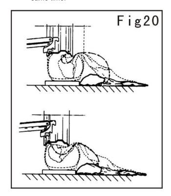
16) Inflate the small amount of air into the tube till without too much folders to guarantee the other side of the tire will not be damaged for the press.
