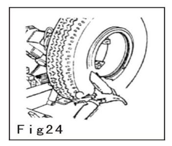
**5**) Move the tool rack to the non-operation position and release the clamp. Move the tire support platform and remove the wheel safely.
