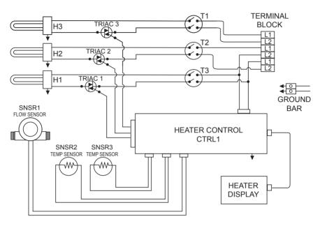
T1, T2, T3 = Thermostat H1, H2, H3 = Heating Element SNSR2 = Inlet Temperature Sensor SNSR3 = Outlet Temperature Sensor
