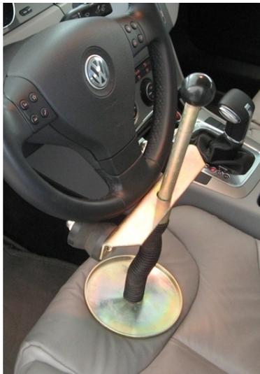
The steering wheel holder holds the steering wheel in position and locks the wheels.
