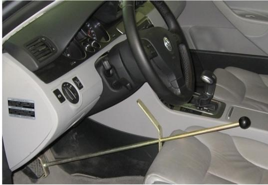
Place a cloth underneath the depressor to protect the seat if necessary. After run out compensation, install the brake depressor for further measurements.
