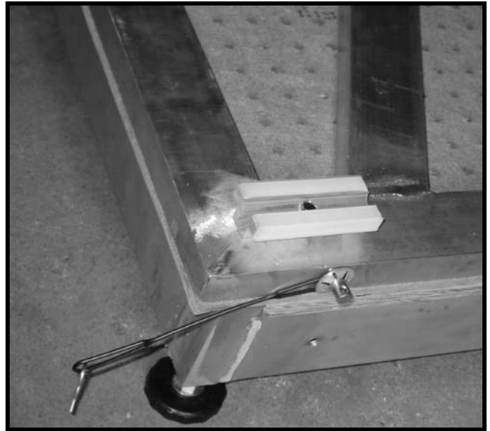
Upper lift shoe placement with clevis pin and lanyard.
