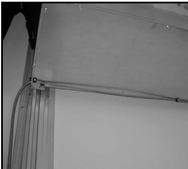
Control cable mounting clip placement on bottom of Loft-it®. Latch bar and protective corner pad installed.
